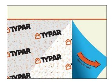
Continue unwinding roll, removing release liner and repeating hand pressure application until course is firmly applied to sheathing. For best practices, use a J-roller or other application tool to ensure any remaining wrinkles and air bubbles are removed from the course.
