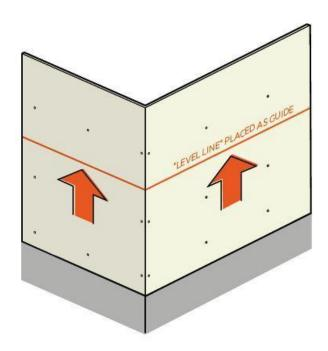
Start at the bottom of one end of the wall with the side without fiber facing up. When starting at a corner, overlap by a minimum of 6" (152 mm). A minimum of a 1" (25.4 mm) overlap on the sill plate is required; however, for maximum protection, a 2"-4" (51–102 mm) overlap on
